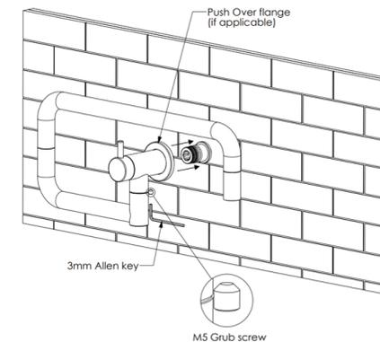
6. Place a bucket or container under the end of the tap spout. Open both cartridges on the tap and switch on the supply water and allow it to flow through the tap for 5-10 seconds. Close each cartridge one at a time (the primary handle is located on the main body of the tap, and the secondary handle is located at the end of the spout) to ensure everything is functioning properly.
