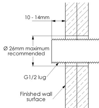
3. Remove any debris or tile glue from the threaded lug and apply thread tape or approved thread sealant to the thread. Using a 12mm hex wrench, thread the brass adaptor over the lug and screw it up until it contacts the finished tile or wall surface. **Do not use vice grips** otherwise the O-rings may be damaged causing leaks. It is important that the brass adaptor is stiff to turn as this is required for the tap stability. If needed, remove the adaptor and apply more thread tape etc.
