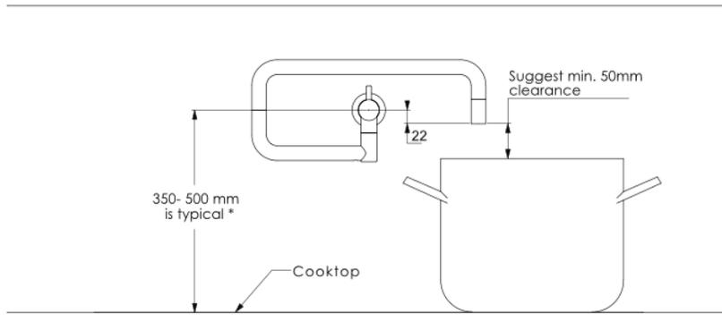
\*The water supply point must be determined and checked by the builder in conjunction with the client. Depending on the application and pot sizes, the ideal mount height can vary significantly from one installation to another.
