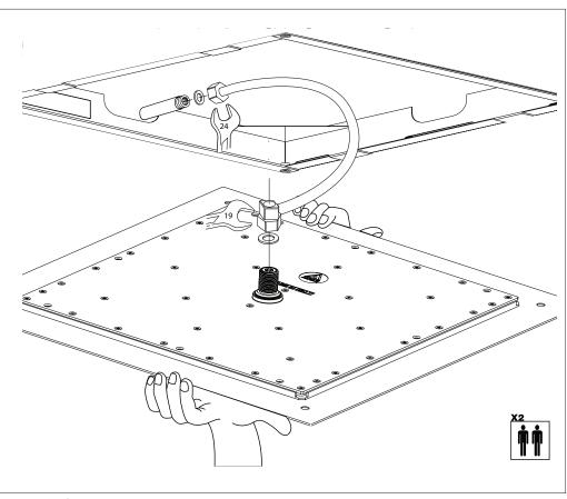
Connect the flexible hose to the water supply line and the shower head as shown, making sure to install the rubber washers provided.
