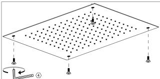
Using an allen key, securely fasten the provided four screws, making sure to tighten them completely.
