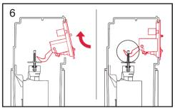
Replace the splash guard. The actuating hooks must be correctly seated in the towing eyes of the drain valve. Tighten the clamping screws of the splash guard.
