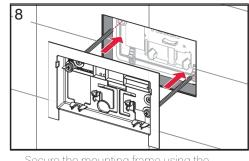
Secure the mounting frame using the fixings supplied.
