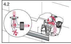
Close the corner valve again and connect the reinforced hose to the filling valve. If you wish to fill the cistern with water the corner valve must then be opened again.
