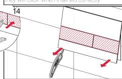
Use the lever supplied to remove the flush plate.
