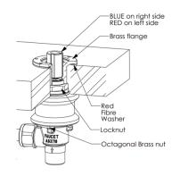
7. Place the Dress Rings over the Brass Flange as shown and align so that the H and C symbols are facing forward (H on the left-hand side and C on the right-hand side). Note that the dress ring has two 'C's – use the appropriate one which faces the correct way for hob installations. Loosely attach the Dress ring using the 3 Cap head screws provided.
