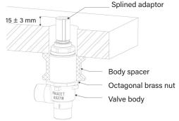
4. Push the Valve body assembly through from the underneath of the basin or sink so that the splined adaptor protrudes through the cut-out as shown above. Adjust the octagonal nut position so that the splined adaptor protrudes above the finished top surface by 15 +/-3mm. Do this for both valve body assemblies (Left and Right sides), Ensure the RED marking is on the left side, and the BLUE marking is on the right side.
